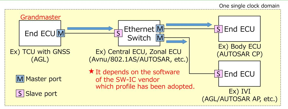
JASPAR assumes that the time synchronization under an environment where various communication software is used together on the same time-synchronization domain.
