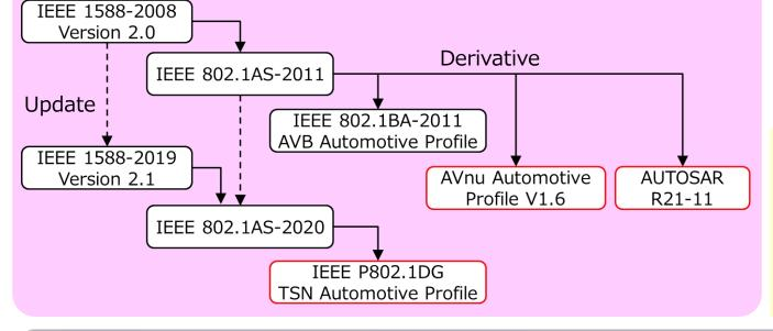
If the profiles for automotive are <u>not</u> <u>consolidated</u>, ECUs based on various profiles will be used together.
