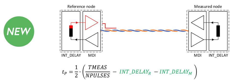
To calculate the propagation delay of the line (t<sub>P</sub>), we need to know the duration of the internal delay (INT\_DELAY)
