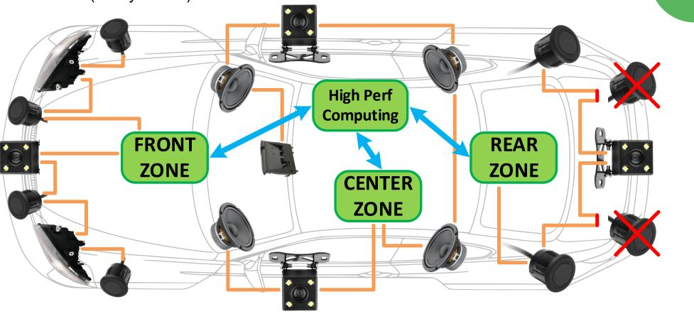
• Enables network flexibility and scalability by distance measurement compared to sequential node ID assignment (allows removing or adding nodes without side effects)
