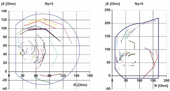
Figure B.8—Examples of equivalent impedance areas based on a set of system conditions
